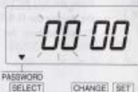
Press the [SELECT] button and position the **▲** mark at the "PASSWORD". The first two digits flash.
