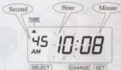
Press the [SELECT] button and position the  $\blacktriangle$  under the "TIME" mark. One can see that the "hour" flashes. (the flashing means that the number can be changed.)
