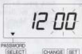
In case of the example, press the [CHANGE] button to select "12", and press the [SET] button. The flashing changes to the last two digits.
