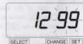
In the example, press the [CHANGE] button to set at "12". And then press the [SET] button.
