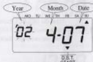
Press the **SELECT** button and position the **▲** over the D.S.T. START. At that moment, the "Year" flashes.
