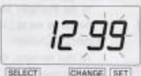
In case of the example, press the **CHANGE** button to set at "12". And then press the **SET** button.
