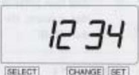
In case of the example, press the **CHANGE** button to set at "34". And then press the **SET** button.
