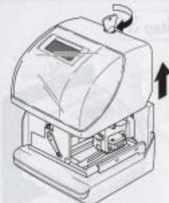
Unlock the key and remove the cover.
