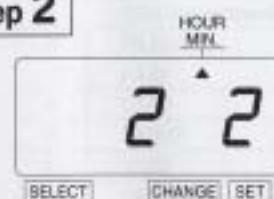
In case of the example, press the [CHANGE] button to set at "2", And then press the [SET] button.
