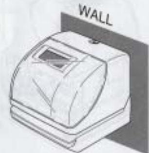
Install the supplied wall-mount screws into a wall by using the template.
