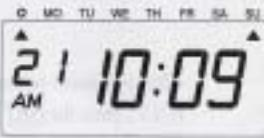
After you finish setting the ending date of D.S.T., press the **SET** button once again. Now the ending date of D.S.T. setting has been completed. Replace the cover and lock.
