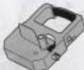
Turn the knob of the new cassette in the direction of the arrow (clockwise) to tighten the ribbon.
