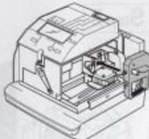
Place the cassette inside the time recorder as shown in the figure. Push the ribbon until it snaps into position. Turning the knob on the ribbon cassette may make installation easier.
